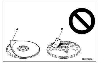
(9) Do not put additional labels (A) or stickers (B) on compact discs. Also, do not use any compact disc on which a label or sticker has started to peel off or any
